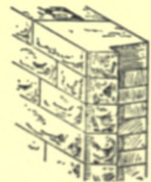
Fig. 35. Window Reveal with Natched Through-stone.
